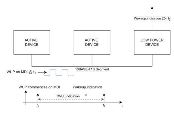
Figure 7-4--TWU\_Indication diagram
