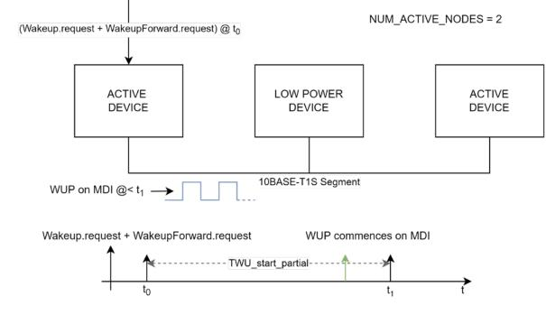
Figure 7-3--TWU\_Start\_partial diagram
