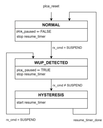
Figure 148-8--PLCA Pause state diagram
