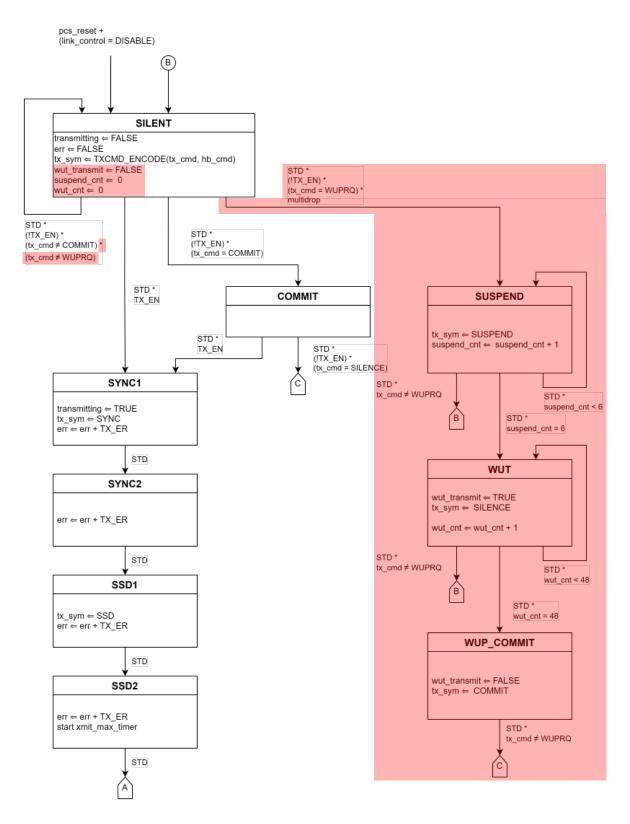
Figure 147-4--PCS Transmit state diagram, part a
