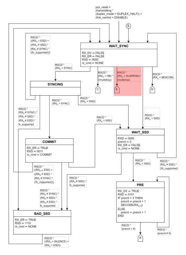
Figure 147-7--PCS Receive state diagram, part a
