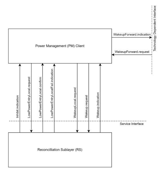
Figure 8-1--Added PM Client and RS interlayer service interfaces
