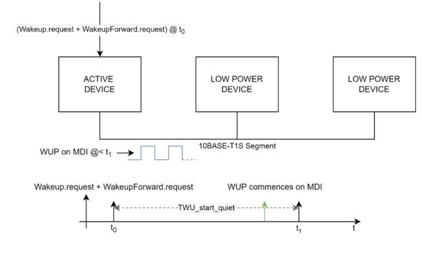
Figure 7-2--TWU\_Start\_quiet diagram
