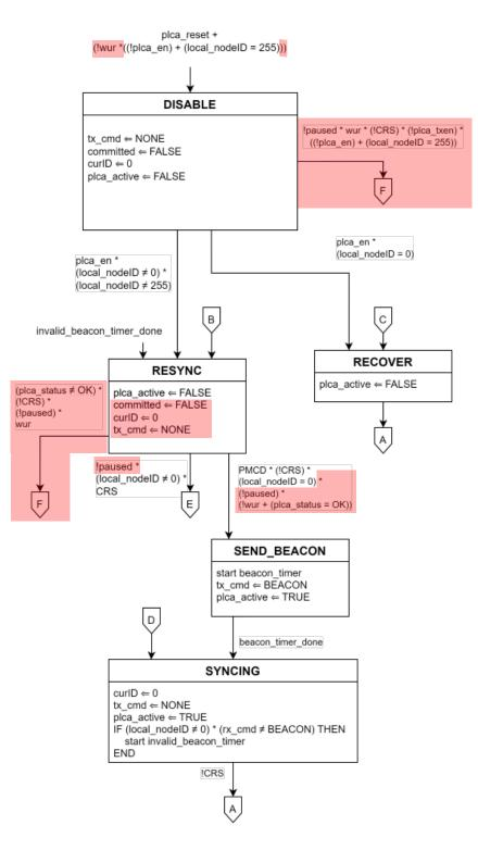
Figure 148-3--PLCA Control state diagram, part a
